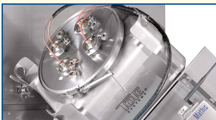
Effusivity pinpoints significant events in your blending process – the end point for optimal uniformity, as well as the onset of de-blending, shear and attrition. If HPLC analysis is required, you can extract correlating thief samples when these critical blend events occur instead of at predetermined times.
