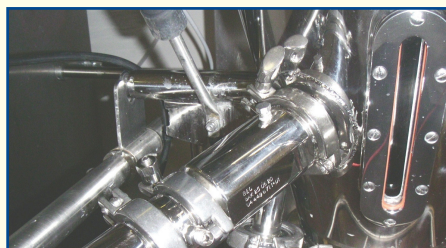
A fluid bed dryer equipped with an ISOLOK™ sampler and ESP sensor provides highly detailed drying profiles and eliminates the need to stop the drying cycle, thief samples, and perform time consuming LOD tests.
